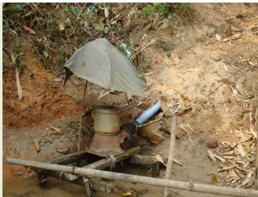
According to Rev. Lazarus, the pipe-fed units are easiest to install. The main requirement is an adequate supply of falling water which can enter a 3-inch intake pipe at a 45-degree angle (although he says, from experience, angles as low as 20 degrees are still usable).
