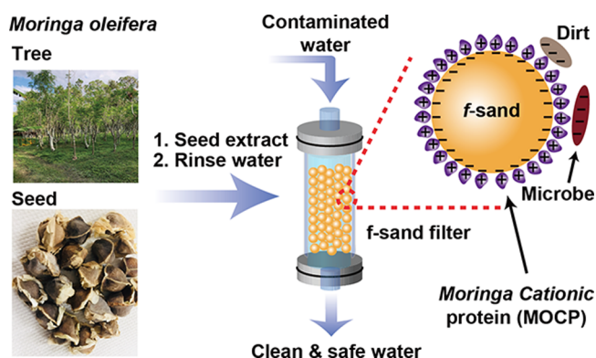
Figure 1. Moringa seed extract-functionalized sand filter ( f -sand) for enhanced pathogen and colloidal removal. Cationic and antimicrobial proteins in Moringa seeds can be readily dissolved and adsorbed onto a sand surface, reversing the charge of the sand particles. These f -sand particles can then be packed into a filter with improved hydrodynamics enabling superior log removal of pathogens. This enhanced sand filter is based on locally available materials and provides an attractive water sanitation option for resource-poor settings.
