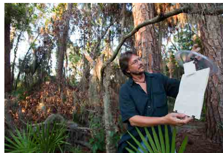
Figure 10. Pheromone trap. Source: USDA, Creative Commons Attribution License
