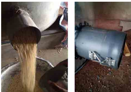
Figure 11. Grain outlet spout and outlet locking lid. Source: Edward Martin
