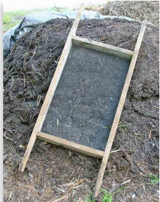
Figure 7. Compost/media sifter made with hardware cloth. Source: ECHO staff
