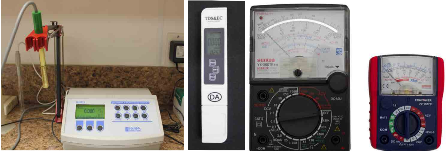
Figure 7: Salinity measuring devices. Shown here are laboratory (left) and hand-held (middle) electrical conductivity meters, as well as ohm/volt multimeters (right). Source: Tim Motis
