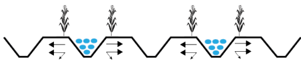
Figure 3: Illustration of "permanent skip furrow irrigation," a raised-bed approach to minimizing root exposure to high salts. Arrows indicate direction of salt movement in response to irrigating every other furrow. Irrigated furrows are indicated with blue dots; non-dotted furrows are those that are kept dry. (Adapted from Devkota et al. 2015)
