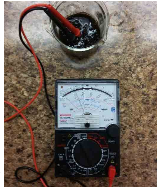
Figure 11: Reading being taken with an ohm/volt multimeter. Source: Tim Motis
