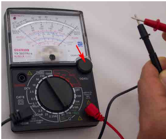
Figure 10: Needle set to zero (right) by turning the zero control knob (see arrow) while touching the red and black lead tips together. Source: Tim Motis
