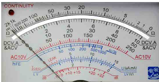
Figure 12: Meter scale of an ohm/volt multimeter. The ohms ( \Omega ) scale is at the top. Source: Tim Motis
