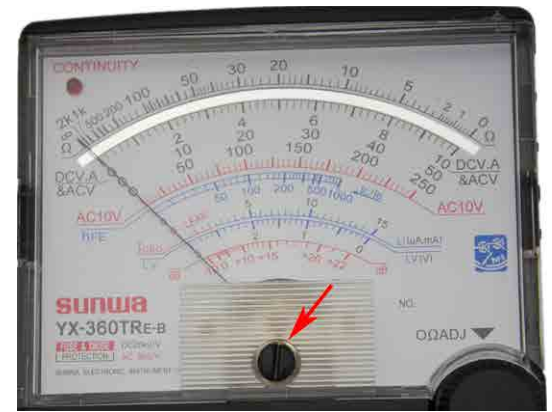
Figure 8: Needle resting on infinity with meter not in use or in the off position. The zero adjuster, as shown by the arrow, can be turned to adjust the needle position. Source: Tim Motis
