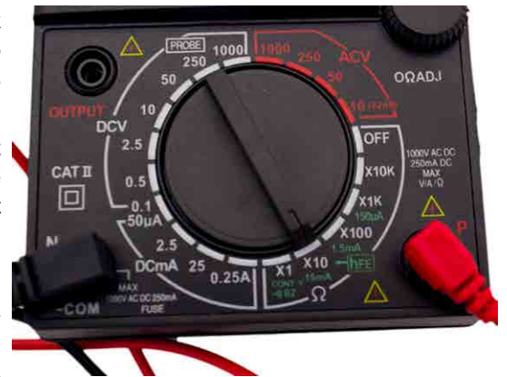
Figure 9: Probe leads connected to the meter set at X10 ohms. Source: Tim Motis
