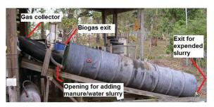
Once this unit is established, it provides a continual supply of biogas and slurry fertilizer. It is estimated that this 3-drum unit could produce about 27 cubic feet of biogas per day and that 2 cows or 10 pigs could supply sufficient manure.
