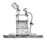
the first week before trying to ignite the stove to assure that there is no air left in the system. This is critical because oxygen mixed with methane can be dangerous if ignited.
