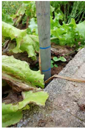
Figure 3. Close-up of soil corer showing depth markings
