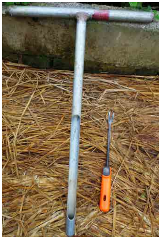
Figure 2. Soil corer for soil sampling (fabricated in a machine shop in Chiang Mai)
