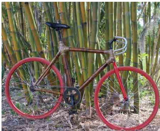
Figure 2. A bicycle from bamboo! Source: Craig Bielema, who built the bicycle from the clump of bamboo growing in the background of the photo.
