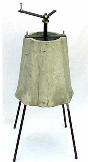
Figure 1: A picture of the Malian peanut sheller. More photos are available on the web (see web address elsewhere in this article). Photo used with permission.
