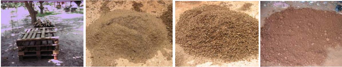
**Plate 2 : From left to right, views of recuperated wood palletes, rice husks, groundnut shells and gravels**
