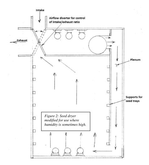
Each light bulb contributes heat to the chamber, and each bulb has a separate switch so that you can control the amount of heat produced. The fan is controlled by a separate switch. Do not make the top cover or doors overly tight. Air leakage (escape) is necessary for circulation, which helps control the humidity.
