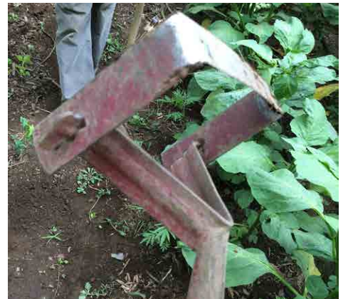
Figure 11. A type of scuffle hoe called a “stirrup” or “push and pull” hoe, this one made in Tanzania. Source: Stacy Reader
