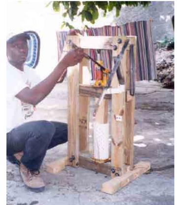
**Figure 5:** Using a press to compress briquettes
