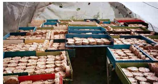
**Figure 9:** Briquettes drying under clear plastic
