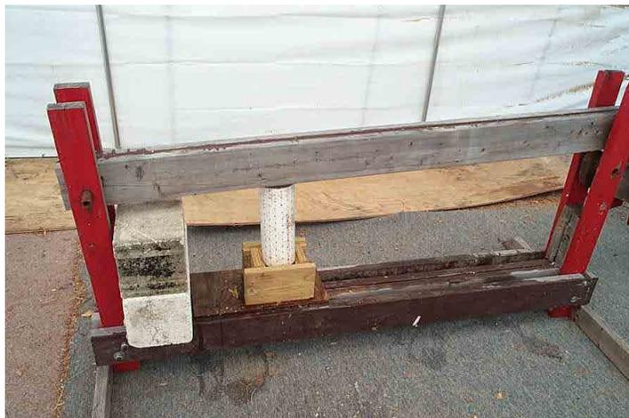
**Figure 18:** Using the press to remove the briquettes from the mold
