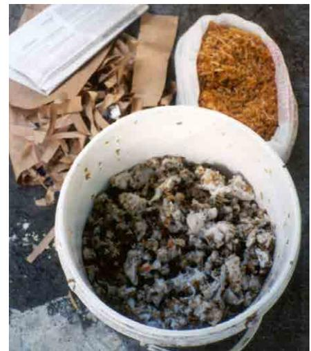
**Figure 1:** Dry materials gathered for making briquettes, old paper and wood shavings (top of photo). Materials after shredding and soaking (bottom of photo).
