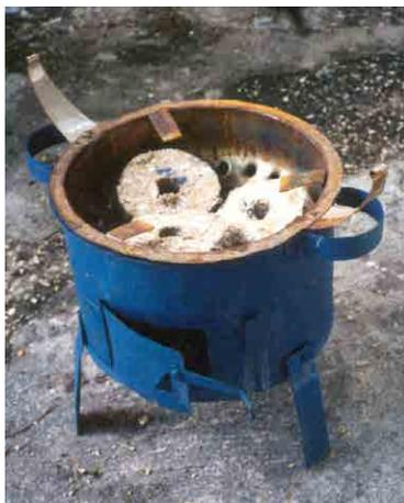
**Figure 10:** Briquettes in a charcoal stove.
