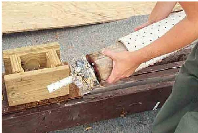
**Figure 19:** Briquette that has been pressed and removed from the mold (center of photo)
