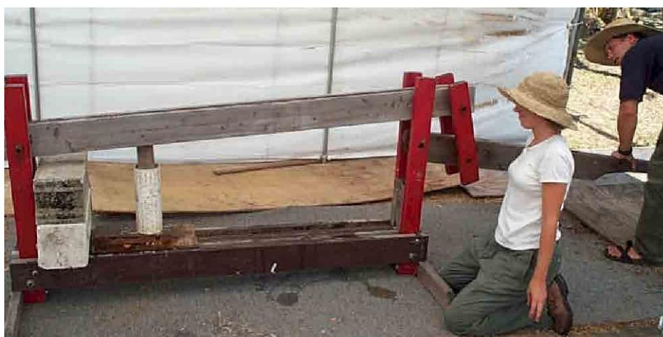
**Figure 17:** Lever arm pushed down to compress briquettes inside mold
