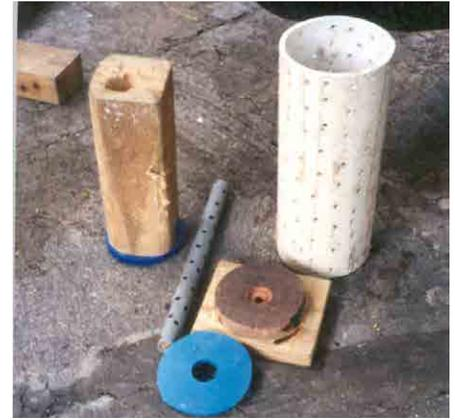
**Figure 2:** (Left to right) Wooden piston, center rod, plastic divider disk, wooden base, PVC cylinder.
