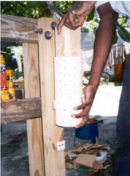
**Figure 6:** Placing mold into extractor, note the PVC square which supports the edge of the mold. Source: Keith Flanagan
