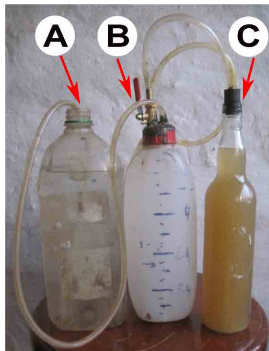
Figure 2. Yeast generates CO 2 in vessel C. This is captured in vessel B and displaces water into vessel A. For CO 2 flushing, vessel C is replaced with a seed-filled storage vessel and water is added to A. This pushes water into vessel B to displace CO 2 , injecting it into vessel C. Source: Thompson, AN 28
