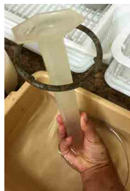
Figure 8. Water displacement method for measuring flow rate of a gas. Source: Tim Motis
