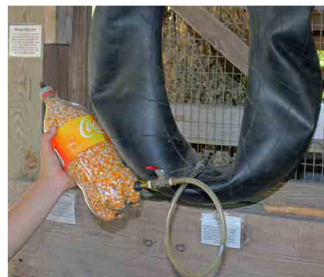
Figure 3. Seed container modified with tire stems at the bottom and top of the seed container. The inner tube was connected to the bottom tire stem, which has its valve core removed to allow gas to flow into the container. The valve core was retained in the tire stem at the top of the bottle so that the valve-core pin could be pressed down (to allow air to escape while the container is being filled with biogas) and then released (to trap the biogas in the container once full). Source: Tim Motis
