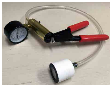
Figure 2. Brake bleeder vacuum pump modified as explained in ECHO TN 93 . Source: Tim Motis
