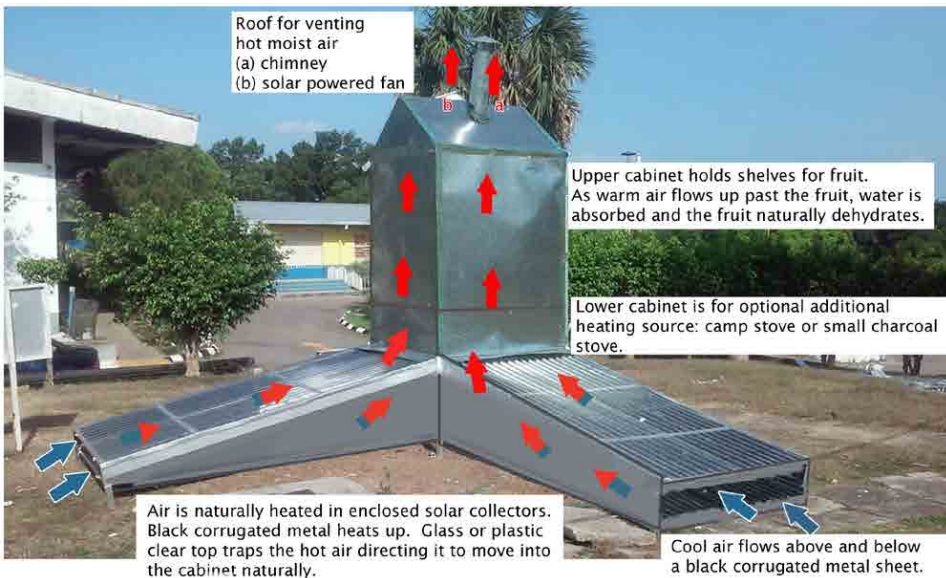
Figure 11. Hybrid solar dryer with arrows showing airflow and parts described. Source: Trees that Feed Foundation ( https://www.treesthatfeed.org/resources/891-2 ).
