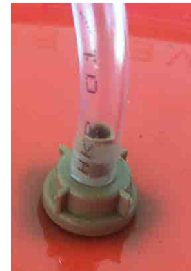
Figure 5. Barbed hose connector on bucket lid. Source: Tim Motis
