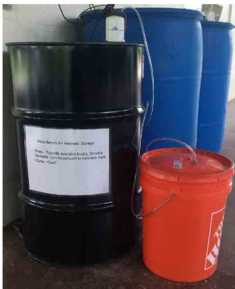
Figure 7. Carbon dioxide from a bucket flowing into a metal drum containing maize seed. Holes for tubing and air escape were drilled into a modified lid, made with PVC plumbing parts, to avoid puncturing the drum. Source: Tim Motis
