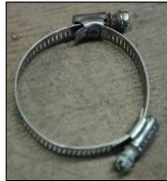
Two hose clamps linked end to end
