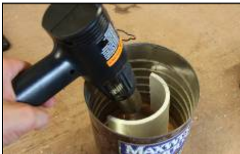
Heating PVC with an electric heat gun
