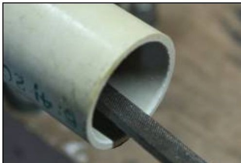
Filing the inside edge of a pipe
