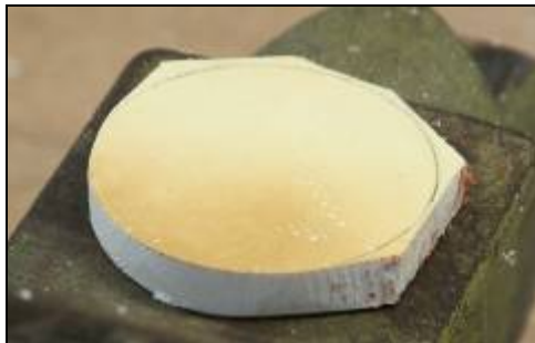
Straight cuts around perimeter of disc, edge filed round
