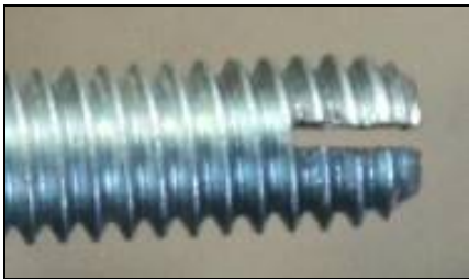
A steel bolt slit at the end, used to tap softer materials
