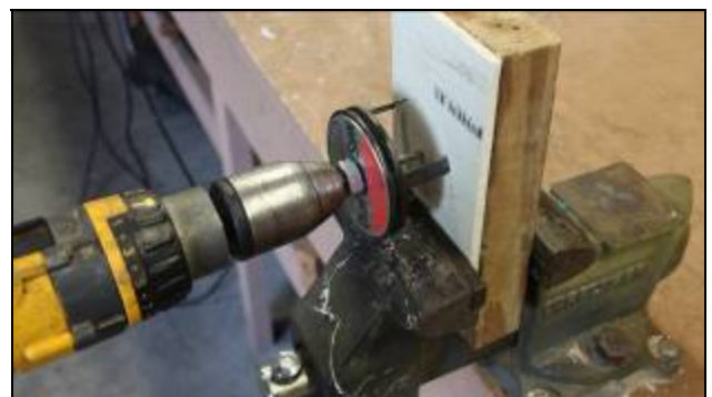
Hole Sawing using a hand drill
