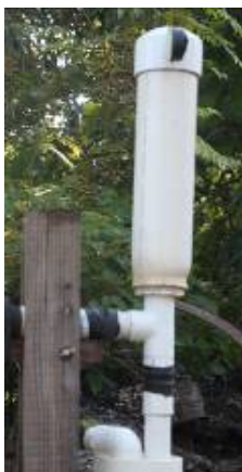
Surge chamber on a rower pump: 4" Sch 40 PVC, 18" long
