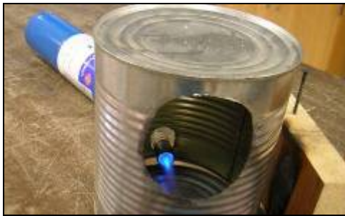
Heating PVC with a torch
