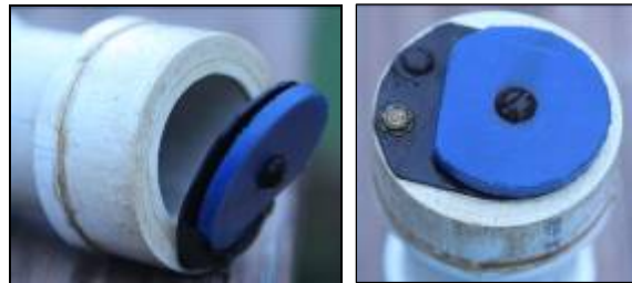
Side flapper foot valve
