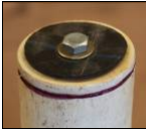
Assembled foot valve
