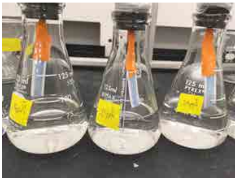
Figure 10. Color of Cyantesmo paper corresponding to 0.25 ppm cyanide. Source: Danielle Hepler
