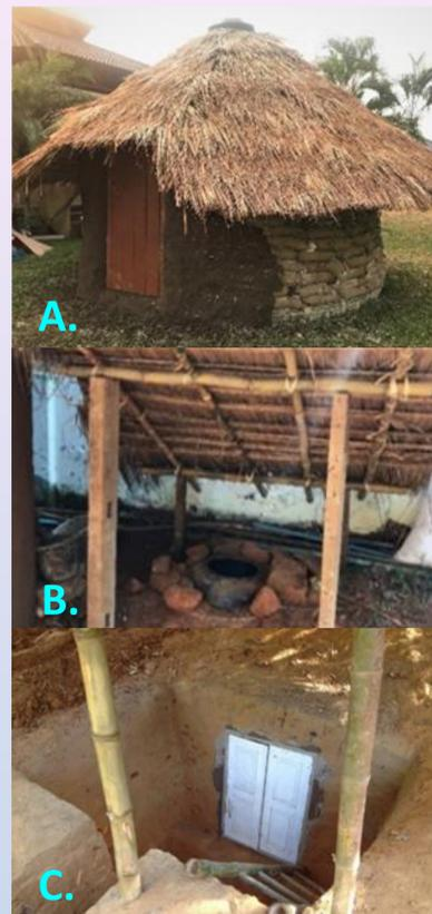
Figure 2. (A) Earth Bag Seed Storage Room. (B) Buried Ceramic Cistern for Seed Storage. (C) Hillside Bunker Seed Storage Room
