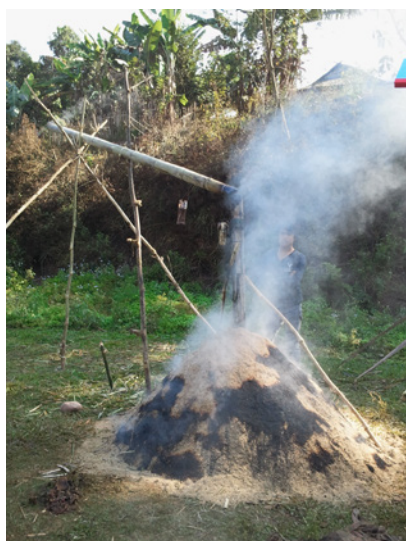
Nearing the end of the charring process (note the wood vinegar collection).
