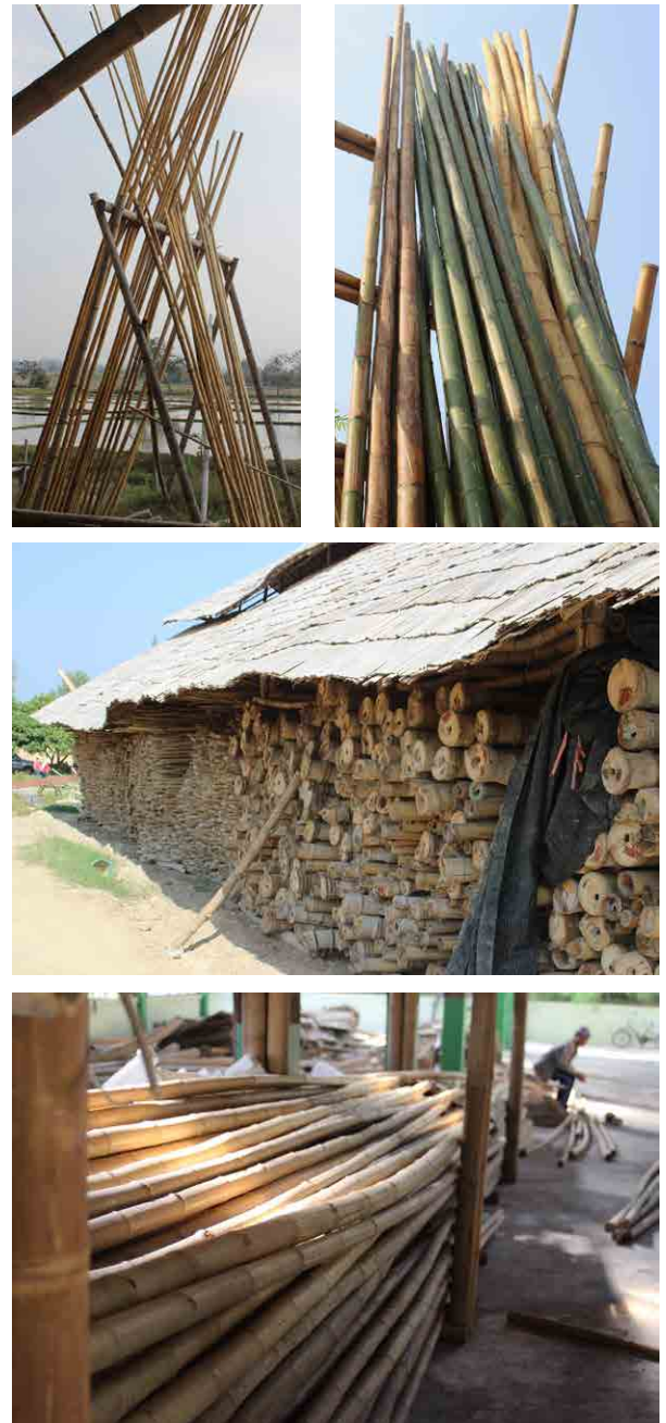
Figure 8. Preserved bamboo drying vertically in the sun (top) and drying and storage racks loaded with bamboo (bottom two). Source: Craig Bielema
