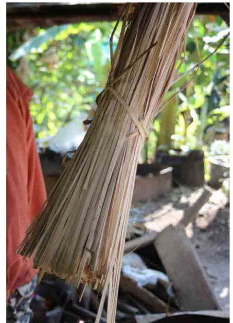
Figure 14. Strips of bamboo bast, to be used for lashing. Source: Craig Bielema
