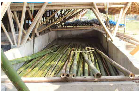
Figure 4. Recently harvested bamboo culms in the process of being preserved by soaking in a tank of chemical solution. Source: Craig Bielema
