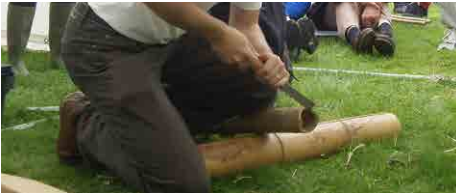
Figure 13. Cutting a fishmouth using a handsaw (top) then Shaping a hand-cut fishmouth using a chisel (bottom). Source: Craig Bielema
