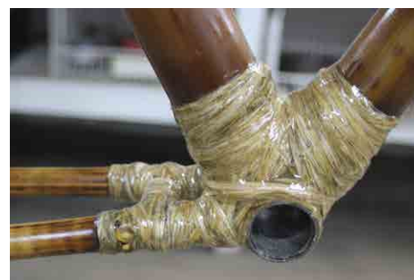
Figure 16. The bottom bracket joint of a bamboo bicycle, held together by a combination of hemp fiber lashing and epoxy. Source: Craig Bielema
