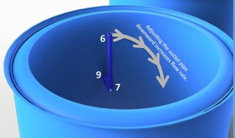
The maximum flow rate through the system is limited by the slow sand biofilter.
