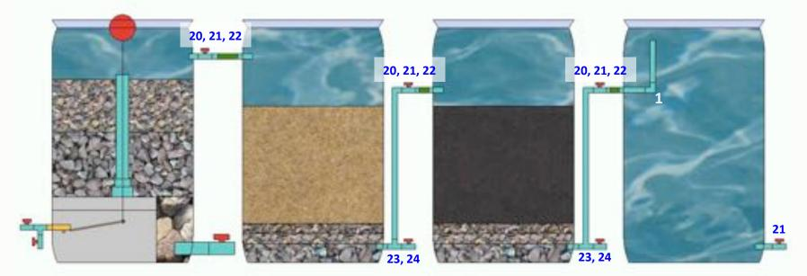
YELD STATE | 1 Fine sand [ 0.1-2.5 mm dia. ] | 2 Crushed biochar [ 1-5 mm dia. ] | 3 Coarse sand [ 2.5-5 mm dia. ] | 4 Pea gravel [ 5-10 mm dia. ] | 5 Coarse gravel [ 10-25 mm dia. ]
