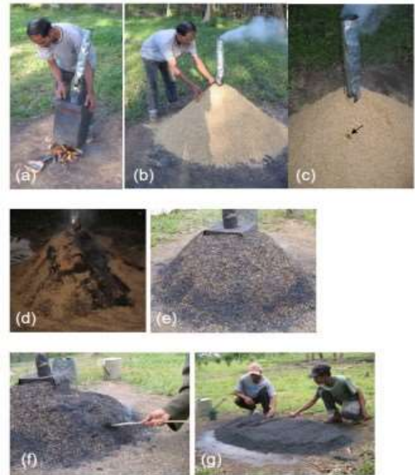
Figure 3.3: The steps of rice hull carbonization. Starting the fire and installing the carbonizer (a), adding hulls to the carbonizer (b), the appearance of carbonized areas on the rice hull pile (arrow) (c), the progression of carbonization (d), the appearance of the pile when approximately 90% of the carbonization has occurred (e), stirring the rice hulls during the final stage of carbonization (f) and spreading out the carbonized rice hulls and halting the carbonization (g).
