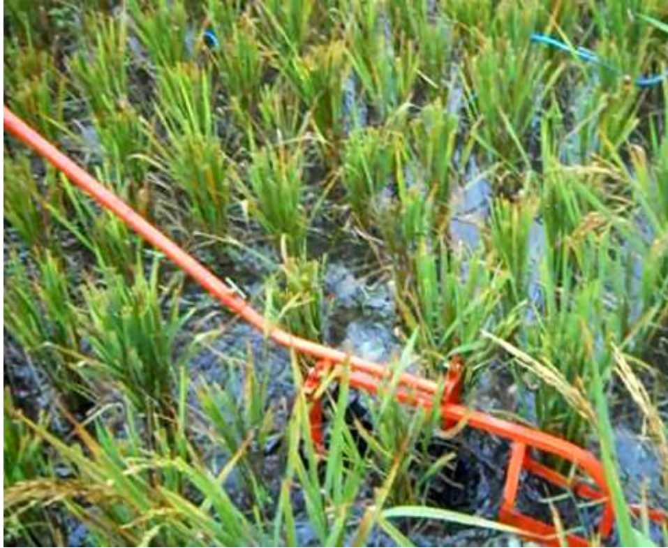
Figure 3. One example of a mechanical weeder with vertical rotating toothed wheels, often used with SRI. Plans are available at ECHO for this weeder and for a larger weeder with five wheels. Sketches of weeders by Paya deMarken, Peace Corps Volunteer in Madagascar.
