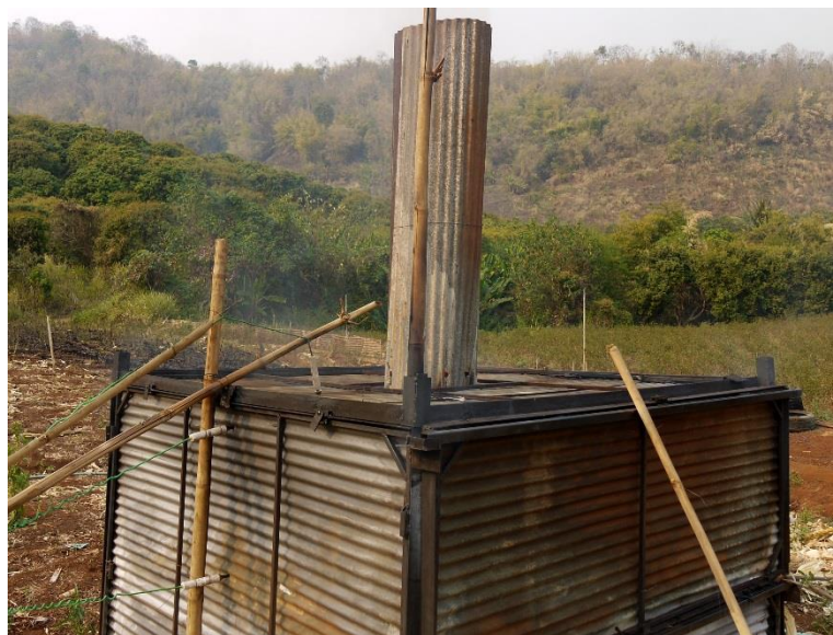
Smokeless, GHG-less pyrolysis of corn stalk into biochar
