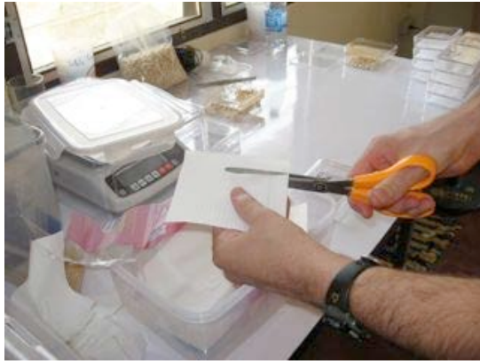
Figure 3: Sizing paper towels for petri dishes: cut a folded paper towel in half with sterile scissors, then trim the long edge of the paper towel to fit perfectly in a petri dish.
