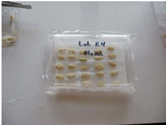
Figure 7: Closed petri dish with plastic bag loosely sealing it and loose edges tucked under (to preserve moisture but allow air exchange).
